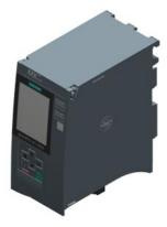
SIMATIC S7-1500F, CPU 1516F-3 PN/DP, central processing unit with work memory 3 MB for program and 7.5 MB for data 1st interface: PROFINET IRT with 2-port switch, 2nd interface: PROFINET RT, 3rd interface: PROFIBUS, 6 ns bit performance, SIMATIC Memory Card required \*\*\*\*approvals and certificates according to entry 109817466 at support.industry.siemens.com to be considered! \*\*\*\*
