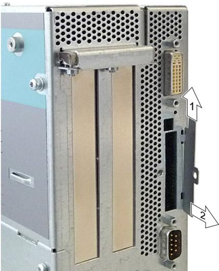
A photograph of the rear panel of a SIMATIC HMI IPC677C. Two white arrows with numbers '1' and '2' indicate the direction to slide the cover plate. Arrow '1' points to the right, towards the DVI connection, and arrow '2' points downwards, indicating the removal of the cover plate. |
