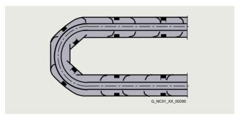
The cables must be able to be moved without applying force, specifically in the bending radii of the carrier.
