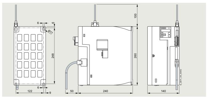
SINAMICS V90, 380 ... 480 V 3 AC, frame size FSC
