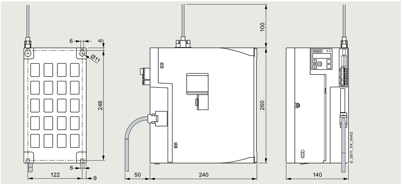
SINAMICS V90, 380 ... 480 V 3 AC, frame size FSC
