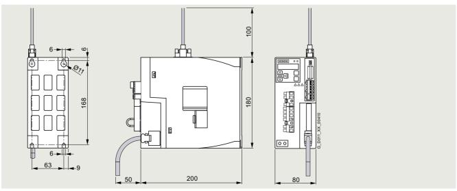
SINAMICS V90, 380 ... 480 V 3 AC, frame size FSA
