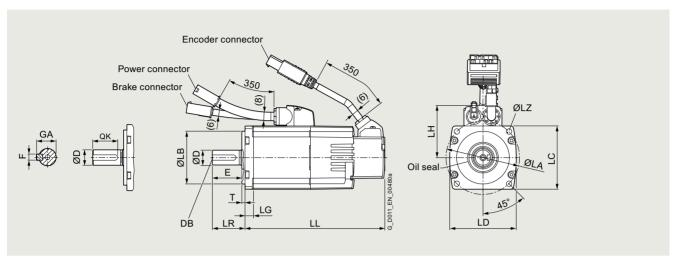
SIMOTICS S-1FL6 Low Inertia servomotors, shaft heights 20, 30, 40
