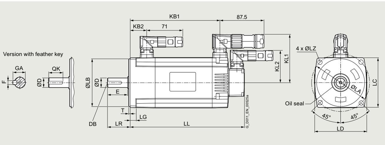
SIMOTICS S-1FL6 Low Inertia servomotor, shaft height 50
