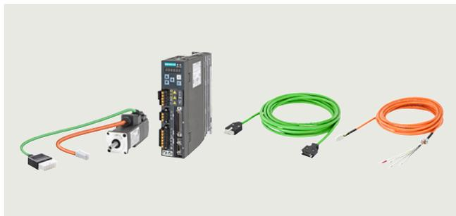
The performance-optimized, user-friendly servo drive system comprises a SINAMICS V90 servo drive and a SIMOTICS S-1FL6 servomotor. There are eight different servo drive frame sizes and seven motor shaft heights for operation on single and three-phase line supplies with power ratings ranging from 0.05 to 7.0 kW, to realize a wide range of applications, with the focus on dynamic motion and processing - for example positioning, transporting and winding.
