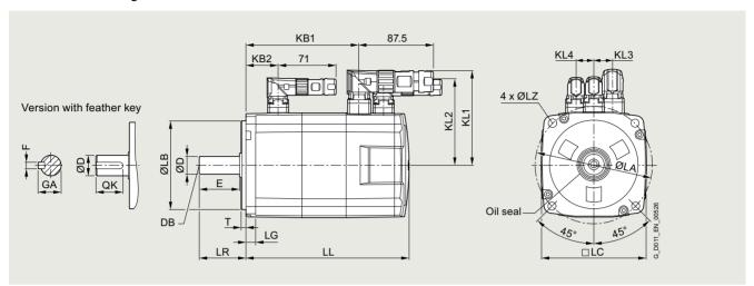
SIMOTICS S-1FL6 High Inertia servomotors, with incremental encoder
