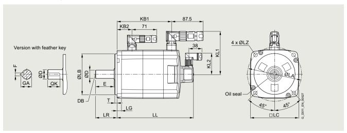
SIMOTICS S-1FL6 High Inertia servomotors, with absolute encoder
