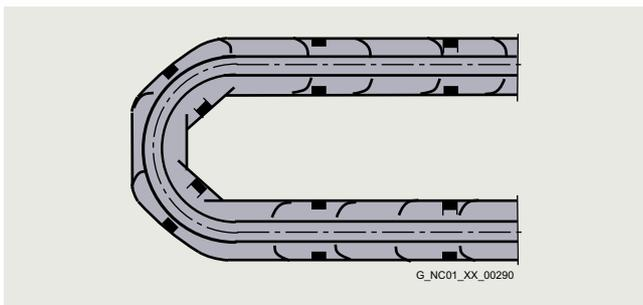
The cables must be able to be moved without applying force, specifically in the bending radii of the carrier. The specified minimum bending radii must be adhered to.
