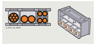
To maximize the service life of the cable carrier and cables, cables in the carrier made from different materials must be separated in the cable carrier using spacers. The spacers must be filled evenly to ensure that the position of the cables does not change during operation. The cables should be distributed as symmetrically as possible according to their weights and dimensions. Cables with different outer diameters should be separated by spacers as well.
