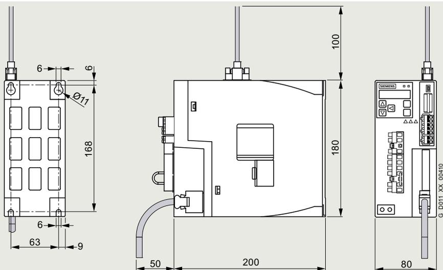
SINAMICS V90, 380 ... 480 V 3 AC, frame size FSA
