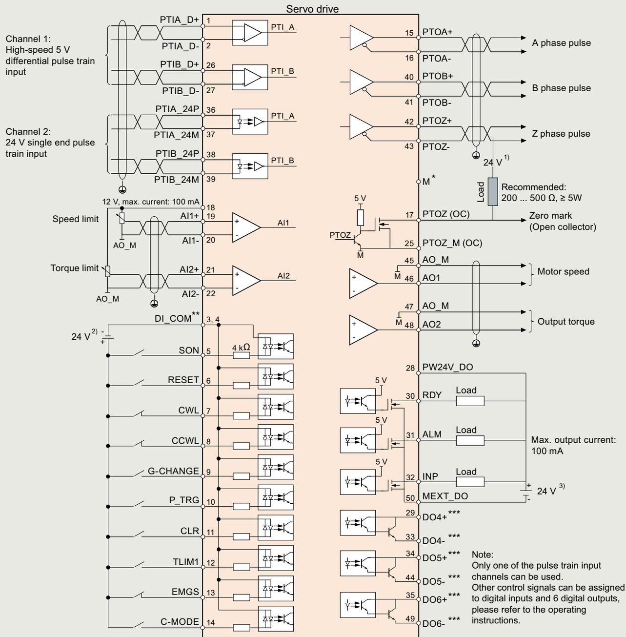
The 24 V power supplies in the connection diagram are as follows:
